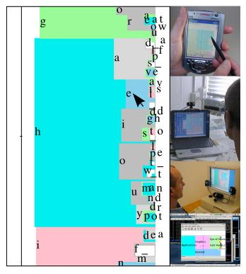
Dasher is a text entry system steered by continuous pointing. Powerful text prediction makes writing easy.
